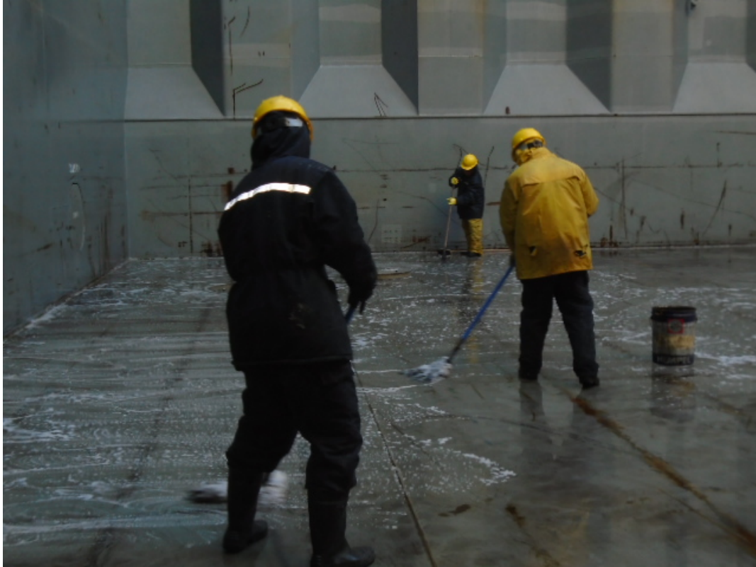
Ship's Crew cleaning tank top with chemical cleaner, mopping and brushing thoroughly
