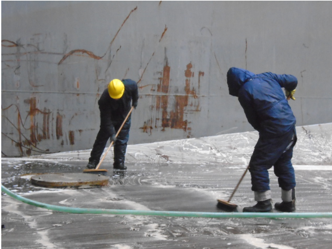
Ship's Crew mopping hatch coaming with chemical cleaner and washing with fresh water
