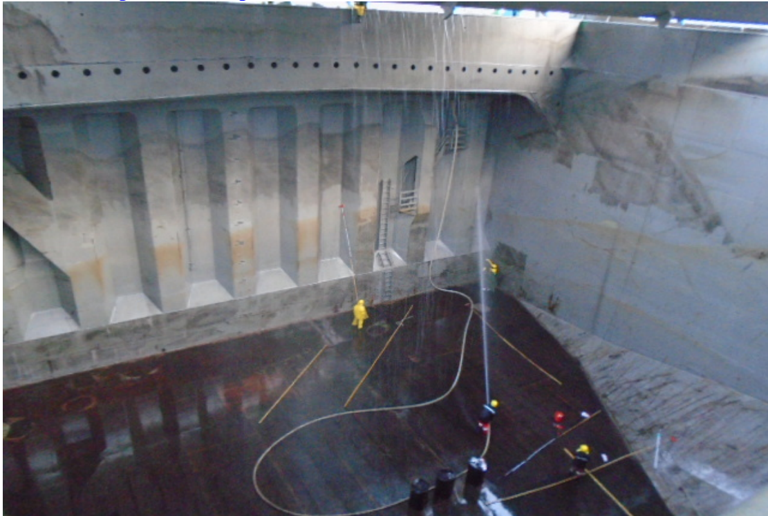
Ship's Crew cleaning the Hold with High pressure machine
